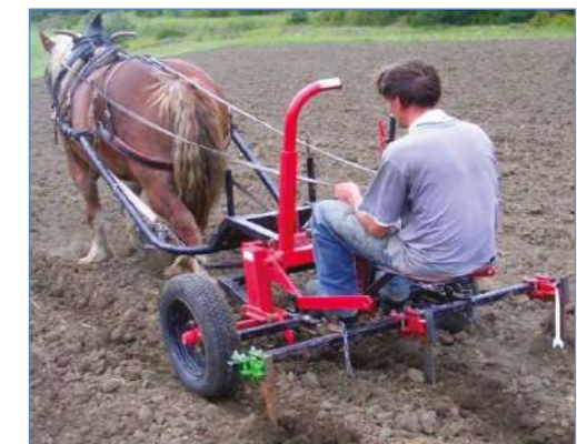
AT tool for soil cultivation and subsequent seeding with constant row spacing
