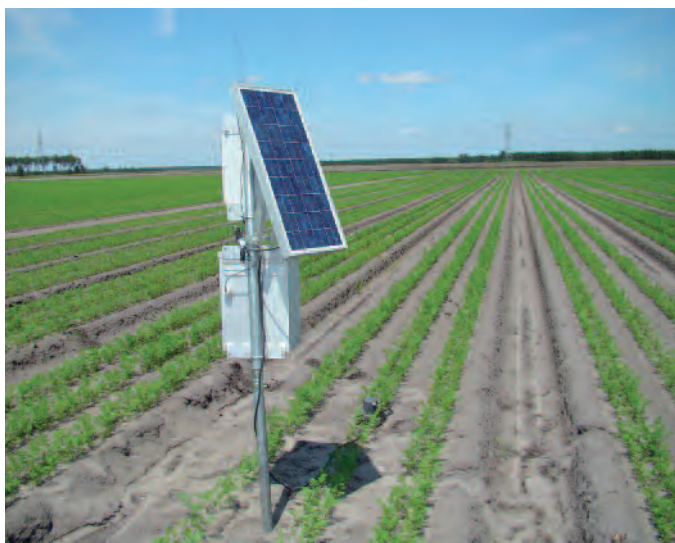
Capacitance probe to measure soil moisture: fine-tuning of irrigation - Gironde (France)
