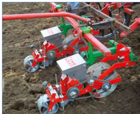
Very solid (but overly expensive) two row seeders allow uniform spacing between rows
