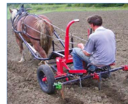
AT tool for soil cultivation and subsequent seeding with constant row spacing
